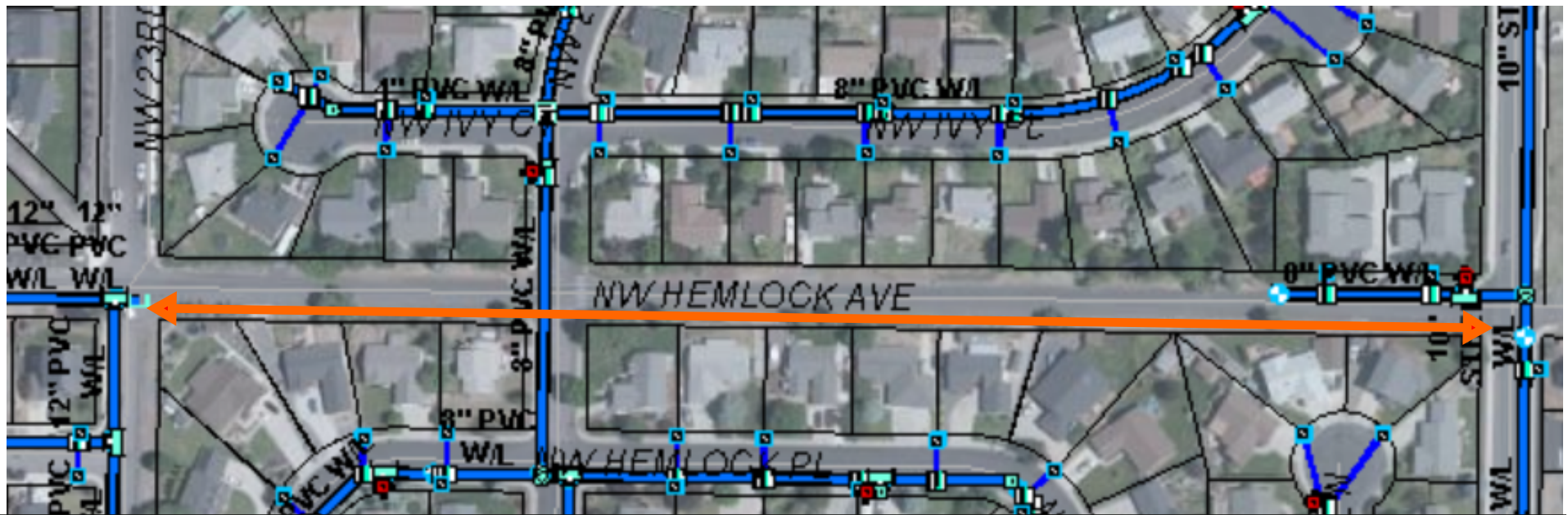
NW Hemlock Ave. from NW 19th to NW 23rd: Complete reconstruction with new curbs, 5' concrete sidewalk on south side, 8' multi-use path on north side, storm drainage, 12" waterline, storm drainage and new pavement and base rock.
