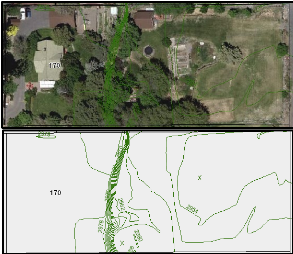
Figure 1 - compact contour lines illustrate defined canyon rim
