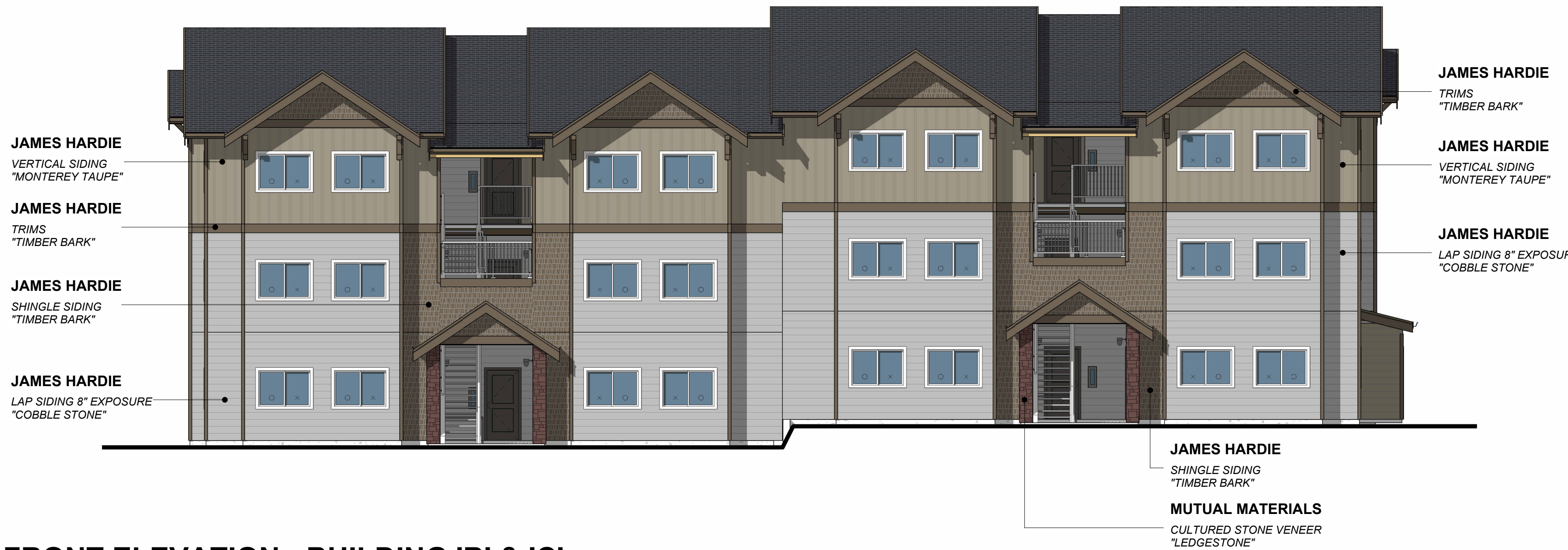
FRONT ELEVATION - BUILDING 'B' & 'C' 1/8" = 1'-0"
