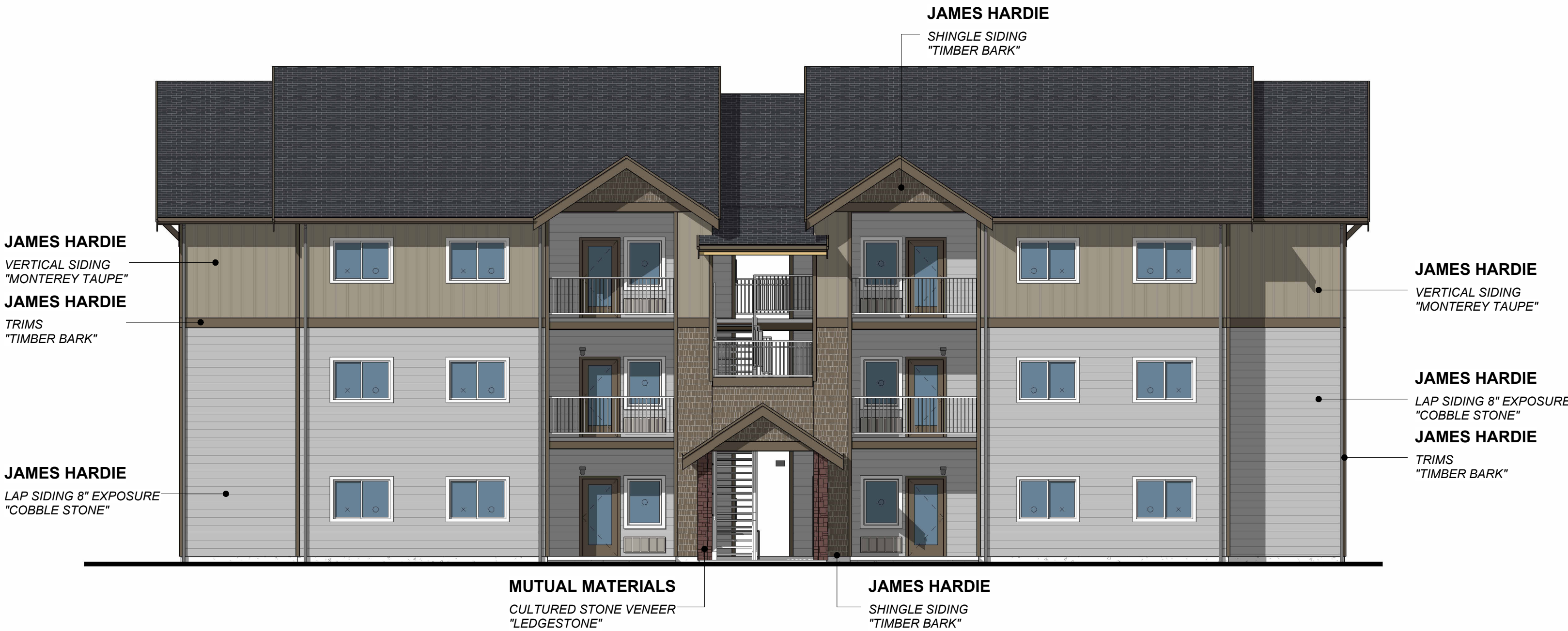
FRONT ELEVATION - BUILDING 'F' & 'K' 1/8" = 1'-0"
