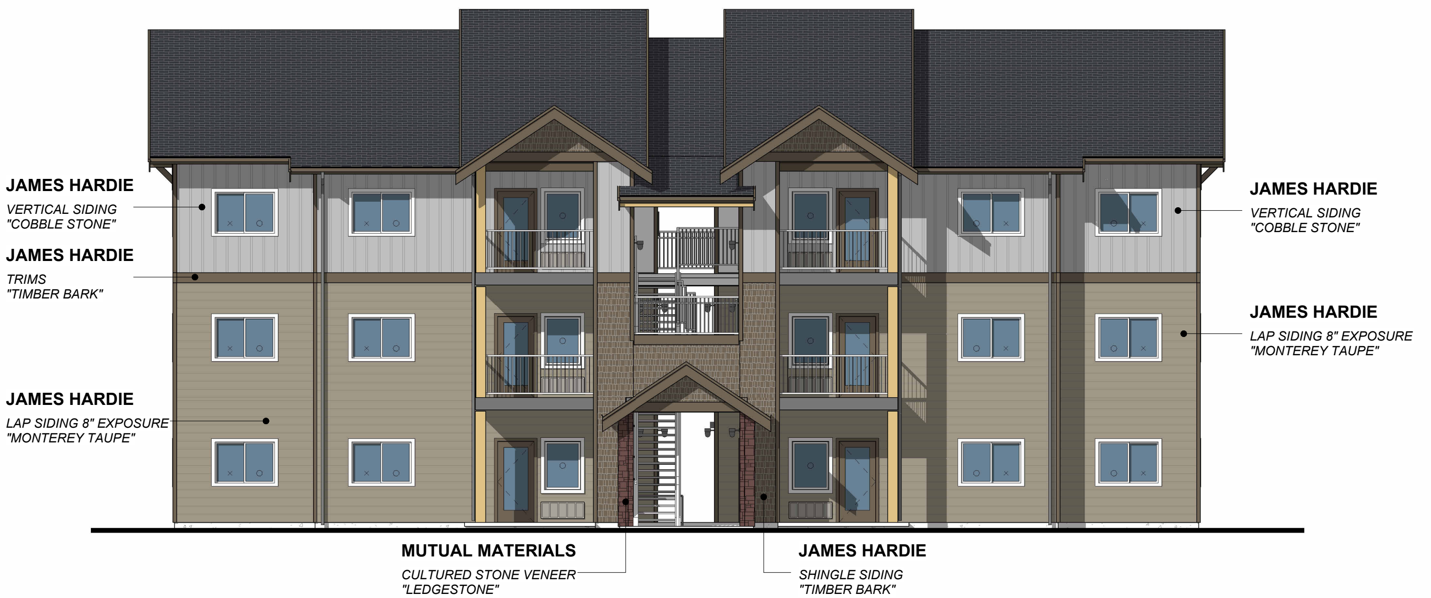
FRONT ELEVATION - BUILDINGS 'J' & 'H' 1/8" = 1'-0"
