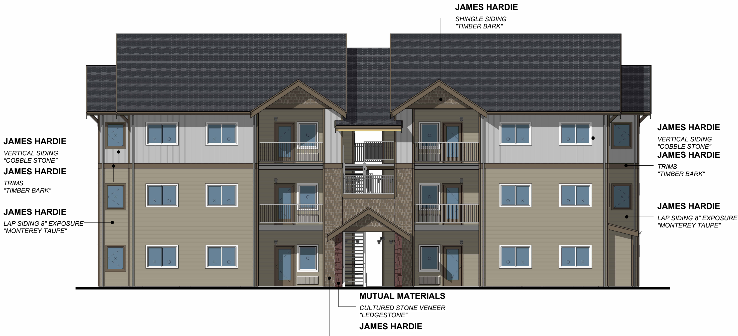
FRONT ELEVATION - BUILDINGS 'A' 'G' 'L' 'M' & 'N' 1/8" = 1'-0"
