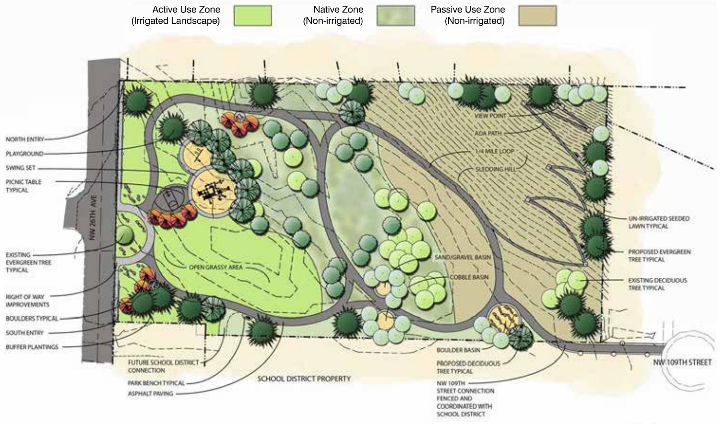
Figure 20. Park Design Schematic Highlighting the Application of Irrigation Zones
