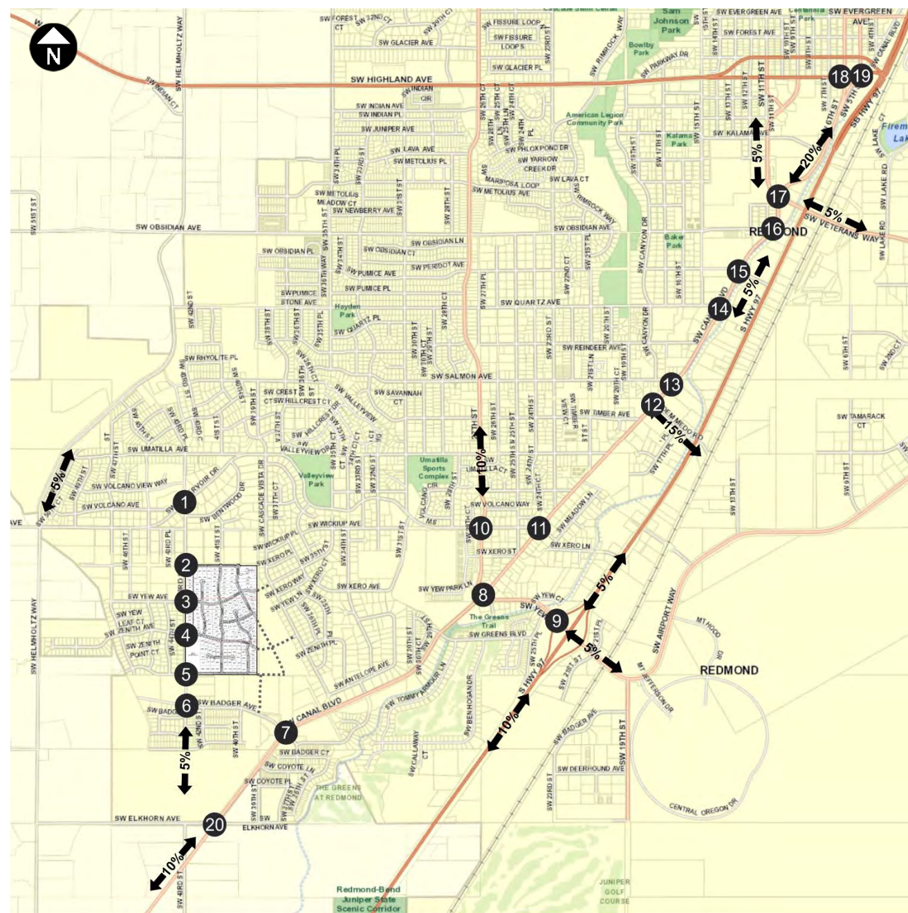
Figure 4. Estimated Vehicular Trip Distribution Pattern and Trip Assignment, Weekday PM Peak Hour. (No 43 rd Street Extension to SW Badger Avenue) Map Source: Deschutes County DIAL.
