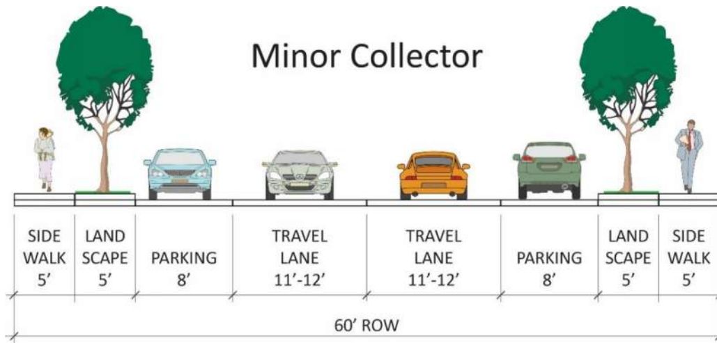
Figure 4: Minor Collector Typical Section
