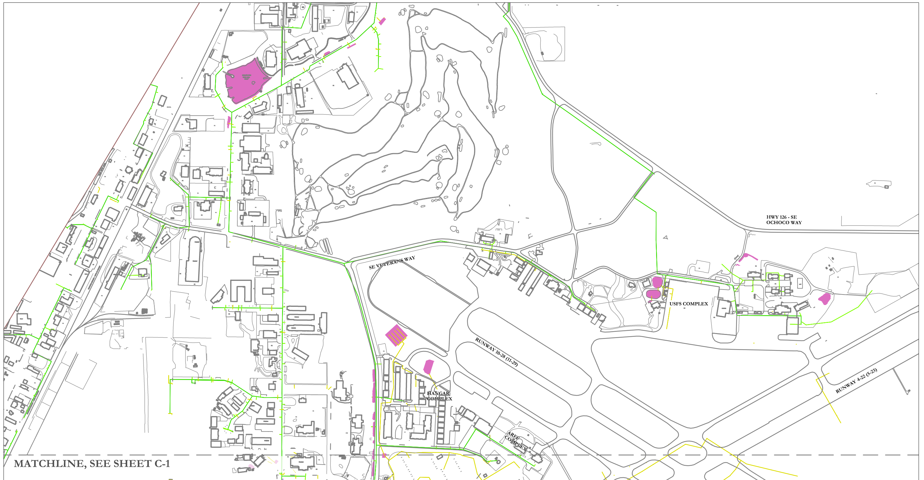
Figure 1-16 EXISTING STORM AND SEWER MAINS AND LATERALS
