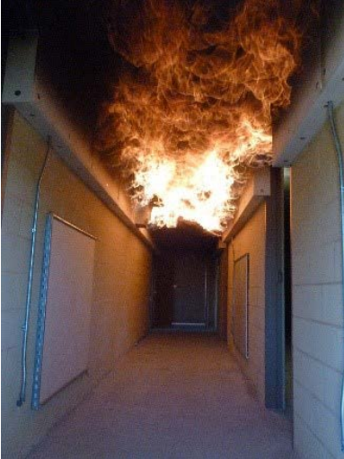
FIGURE 18 - TYPICAL FLASHOVER PROP
