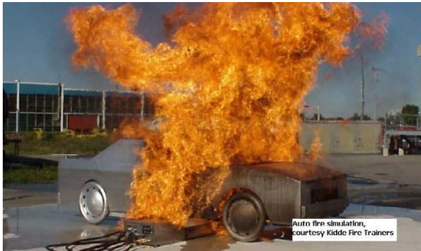
FIGURE 20 - TYPICAL VEHICLE LIVE FIRE PROP
