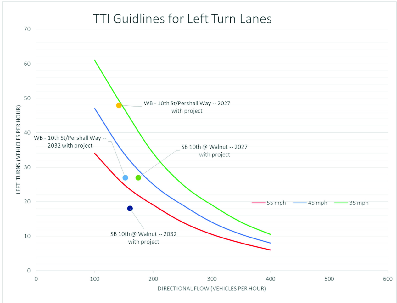
Exhibit 1 Left Turn Warrant for 10 th @ Walnut not met (Speed 35 mph); Warrant met for turn lane on Pershall Way at 10 th in short term but when Upas Bridge is built, left-turn volume was forecast to be lower. In the latter case, warrant is not met at 45 mph, but met at 55 mph. Speed is not posted.
